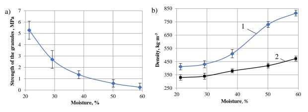
Fig. 4. Dependence of the static strength of the granules (a) and density (b) on their moisture content: 1 – unit density; 2 – bulk density
