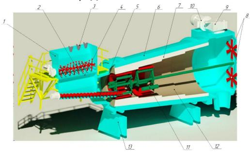
Fig. 1. **3D** model of a machine for production of organic sapropel-based fertilizers: 1 – hopper; 2 – mixers; 3 – dispensers; 4 – valve; 5 – screw conveyor; 6 – drum; 7 – drying surface with ceramic coating; 8 – fans; 9 – reducer; 10 – electric motor; 11 – rollers; 12 – perforated cylinder; 13 – supports
