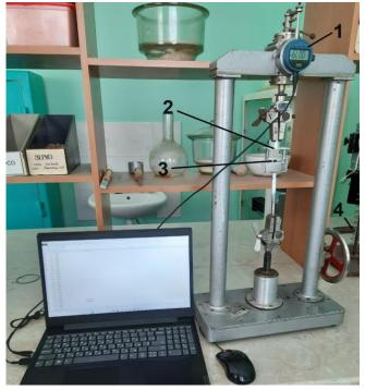
Fig. 3. Picture of the setup for testing the granule strength
